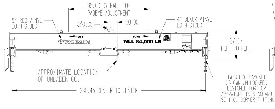
SOULDES ALL HAVE BOLT ON 1/2" THICK UHMW-PE PADS COVERING CONTACT AREAS WITH CONTAINER
