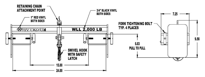
To avoid lifter failure, potential death and property damage, never exceed WLL (Working Load Limit).
