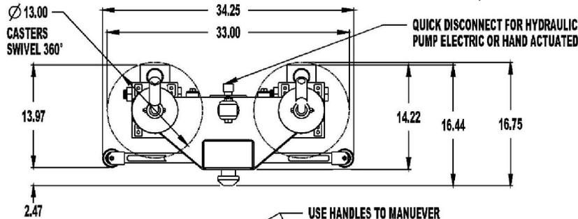
STANDARD SET OF FOUR (P/N: R17000A-1PA) INCLUDES 4 LIFT CASTER ASSEMBLIES, HANDLES (FOR TRAVEL) AND 2 HAND PUMPS WITH 6' HOSES AND QUICK-DISCONNECT FITTINGS. AN ELECTRIC PUMP WITH MANIFOLD AND 4 LINES IS AVAILABLE AS AN OPTION.
