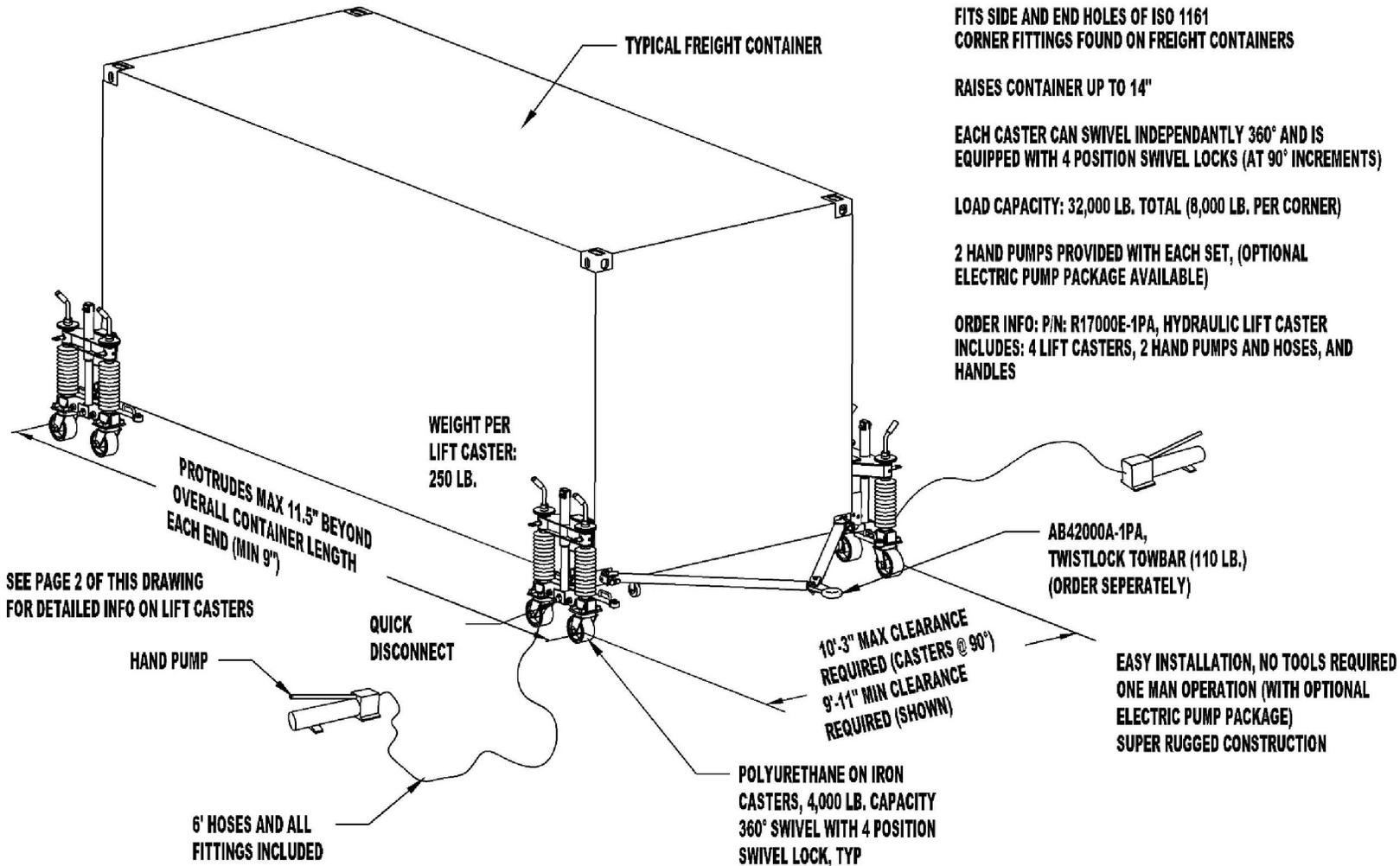
To avoid lifter failure, potential death and property damage, never exceed WLL (Working Load Limit).
