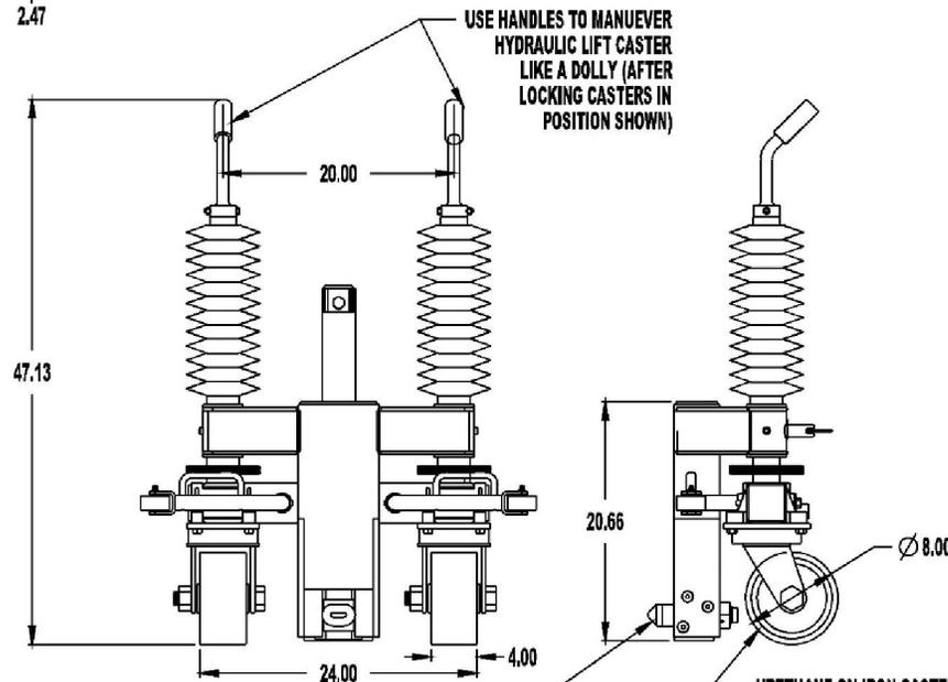
PLUGS IN EITHER SIDE OR END HOLE OF STANDARD ISO 1161 CORNER FITTING. ROTATE 90° TO LOCK, TIGHTENS AUTOMATICALLY AS CONTAINER IS LIFTED. WHEN USED IN SIDE HOLES, TANDEMLOC TOWBAR AB42000A-1PA IS STRONGLY RECOMMENDED FOR TROUBLE FREE TOWING
