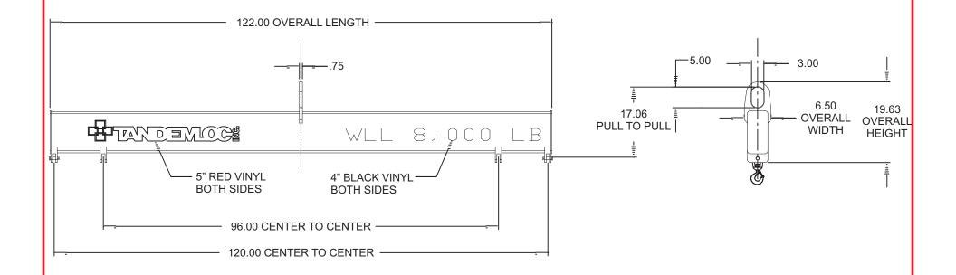
To avoid lifter failure, potential death and property damage, never exceed WLL (Working Load Limit)
