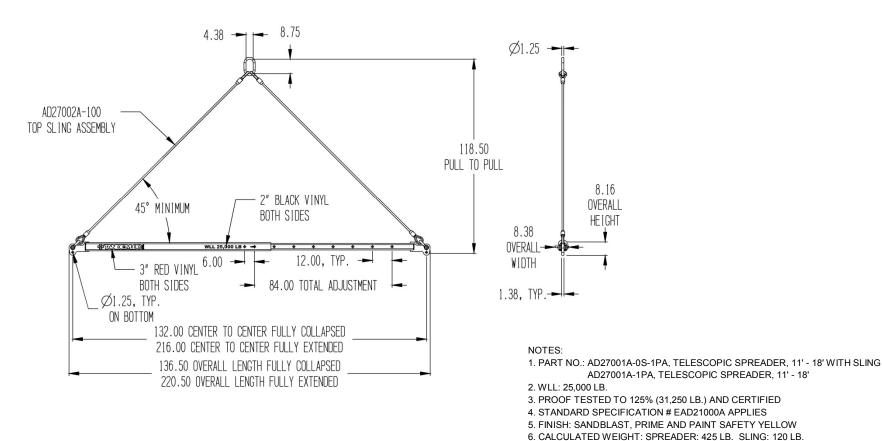
To avoid lifter failure, potential death and property damage, never exceed WLL (Working Load Limit).
