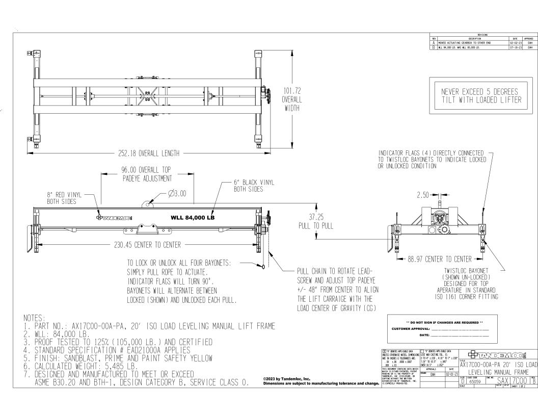
BEFORE LIFTING THE LOAD, THE CARRIAGE SHOULD BE POSITIONED OVER THE CG OF THE LOAD. MINOR ADJUSTMENTS CAN BE MADE WHILE LOADED.
