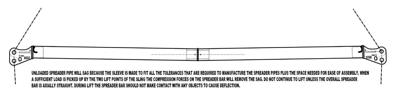
WHILE UNLOADED SAG DOES NOT IMPAIR THE LIFT CAPABILITY OF THE CONNECTION SLEEVES, IF DESIRED, THE UNLOADED SAG CAN BE REDUCED ONCE THE ACTUAL SPREADER PIPE CAN BE MEASURED. THE OUTER DIAMETER OF THE PIPE ENDS CAN HAVE STEEL SHIMS ADDED TO REDUCE SAG BY UP TO 50%. THE SUGGESTED METHOD IS SHOWN IN DETAIL "A". THIS IS AN EXTRA COST OPTION AND IS NOT INCLUDED IN THE PURCHASE PRICES.
