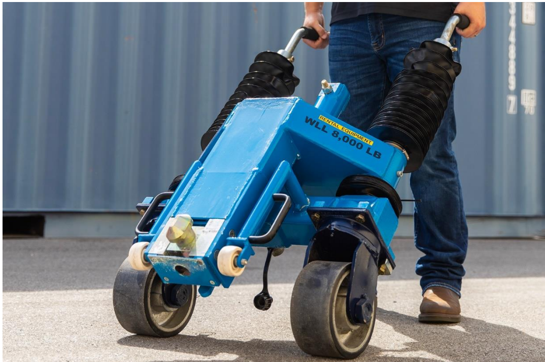
Figure 4.1.1 - Move the Lift Caster into position
