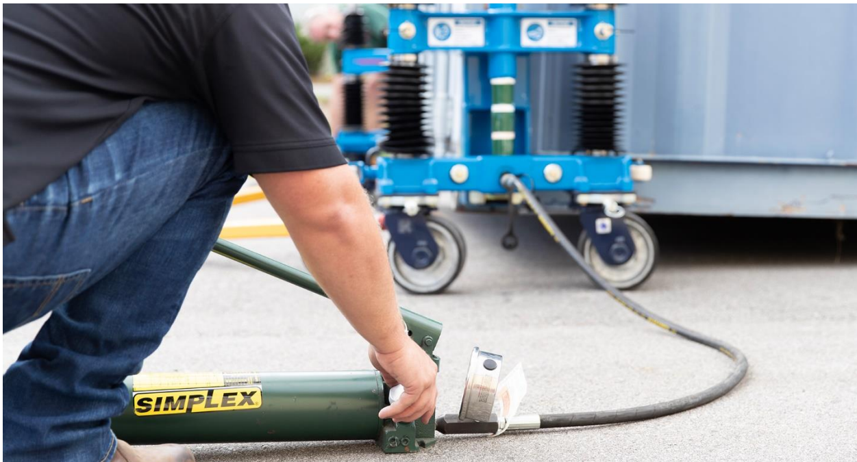
Figure 3.2 - Using the hand pump
