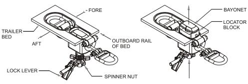
1. HOUSING IS WELDED INTO STRUCTURE AND INTERNAL PARTS ARE ASSEMBLED.\* MAKE SURE STAR SHAPED SPINNER NUT IS AT BOTTOM OF BAYONET
