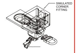
4. LOWER CONTAINER WITH CORNER FITTINGS ONTO BAYONETS AND THEN TURN HANDLE BACK 90°. THE CORNER FITTING CAPTURES THE LOCATOR BLOCK PREVENTING IT FROM TURNING BUT ALLOWS THE BAYONET TO TURN TO LOCK INSIDE OF THE CORNER FITTING
