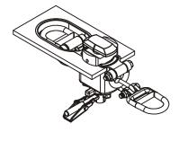
6. WITH THE BAYONET LOCKED INSIDE THE CORNER FITTING, TIGHTEN THE SPINNER NUT UNTIL HAND TIGHT. THE LOCK LEVER WILL NEED TO LINE UP AND EITHER CAPTURE OR BLOCK A SPOKE OF THE SPINNER NUT TO PREVENT IT FROM TURNING EITHER DIRECTION.
