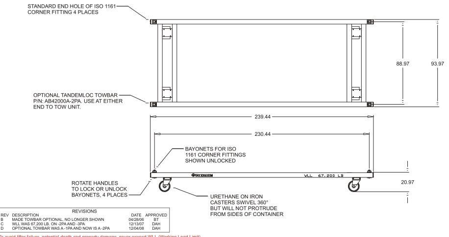
To avoid lifter failure, potential death and property damage, never exceed WLL (Working Load Limit)
