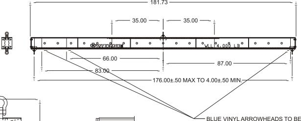
BLUE VINYL ARROWHEADS TO BE MARKED ON BOTTOM FLANGE MARKING THESE THREE POINTS
