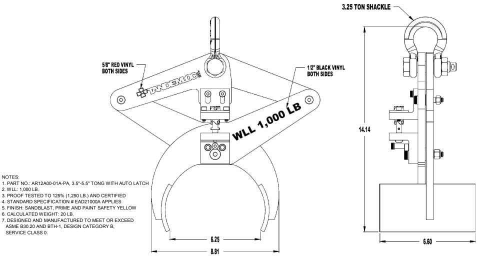
To avoid lifter failure, potential death and property damage, never exceed WLL (Working Load Limit).
