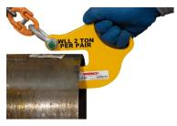
The Tandemloc Pipe Hook lifting system provides a simple, secure and efficient method of lifting and handling pipe sections and pipe-like fabrications or components. The integrated, ergonomically designed handle provides for a safe and convenient method of holding and inserting the pipe hook into the lifted section.
