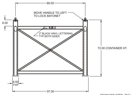
2 TWISTLOCK BAYONETS WITH HANDLE, DETENTS WITH BALL AND SPRING LOCATE THE LOCK AND UNLOCKED POSITIONS FOR ISO 1161 CORNER FITTINGS. (LARGE HOLE) 75.25 84.00
